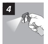
Spray the glass coating from a distance of less than 5 cm from the car's body.
