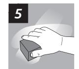
Using a clean, water-dampened, and well-wrung sponge, spread the glass coating evenly in a vertical and horizontal motion without worrying about streaks.
